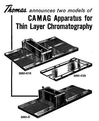
THIN LAYER CHROMATOGRAPHY APPARATUS, **Camag.** For applying uniform coatings of inorganic materials to glass plates for adsorption or partition separation of 0.5 to 500 microgram samples using paper chromatography techniques.
